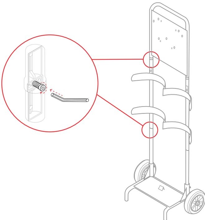
5. Once all parts are in position, tighten all expanders (**A+B**) with an allen key to secure the complete frame.
