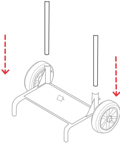
1. Slot the legs of **Part 2** into the short pipes of **Part 1**.
